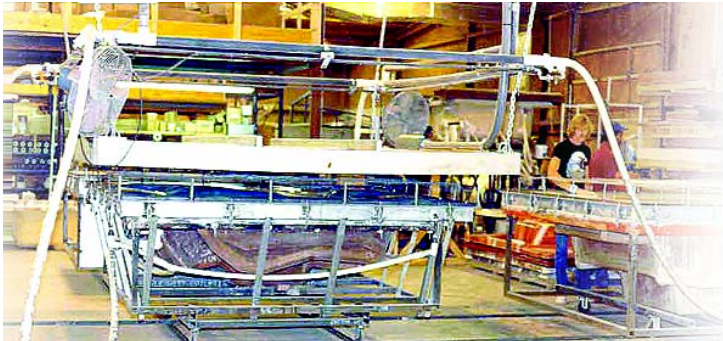
Double Ender quick change molds on wheels four post system
